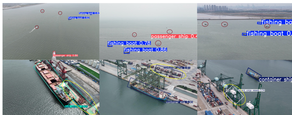
Figure 15. Visualization of false negatives and false positives. Red circles indicate missed detections, while yellow circles indicate false detections.
